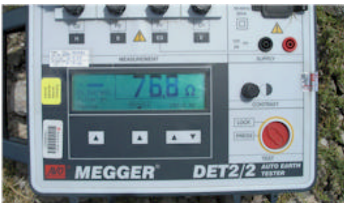
This is a photo showing the final reading of the two installed galvanized plates tied together in a single layer of Poly-Ground® after the trench had been backfilled with soil but not compacted. The final reading was 76.8 ohms.
