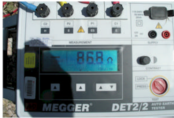
Pole 4: This photo shows the “connecting” of the two plates using a Poly-Ground® only connection and the subsequent reading, keeping in mind there is still only a bottom connection to the earth.
