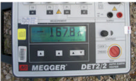
Pole 4: This is the reading of one plate encased in Poly-Ground®. It is important to note the only contact the plate/Poly-Ground® had with the ground was the bottom section as there are no sides and there is no backfill on the top. It is open air. The reading is 167.8 ohms.
