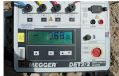
Pole 3: #1 is the ground rod isolated; reading= 10.45 ohms. #2 is the Poly-Ground backfilled plate isolated; reading=13.53 ohms. #3 is the copper rod and Poly-Ground plate tied together; reading= 8.68 ohms.
