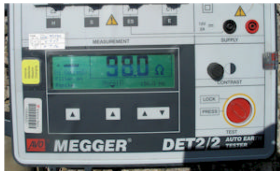
Pole 4: This structure was set on a pre-cast concrete foundation that had a galvanized plate put in the trench but was not treated with any backfill other than native earth. The plate was placed vertically in the trench and backfilled with the excavated material. The reading was 98.0 ohms.
