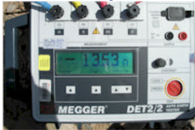
Pole 3: #1 is the ground rod isolated; reading= 10.45 ohms. #2 is the Poly-Ground backfilled plate isolated; reading=13.53 ohms. #3 is the copper rod and Poly-Ground plate tied together; reading= 8.68 ohms.
