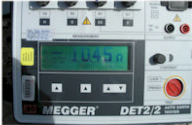
Pole 3: #1 is the ground rod isolated; reading= 10.45 ohms. #2 is the Poly-Ground backfilled plate isolated; reading=13.53 ohms. #3 is the copper rod and Poly-Ground plate tied together; reading= 8.68 ohms.
