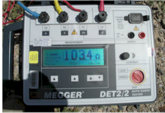
Pole 4: This photo shows the second installation and megger reading was 103.4 ohms. This reading is a cumulative reading of the first plate tied together with the second plate. So there are actually two plates tied together being read here, but there is still only bottom contact being made as the hole is still open air.
