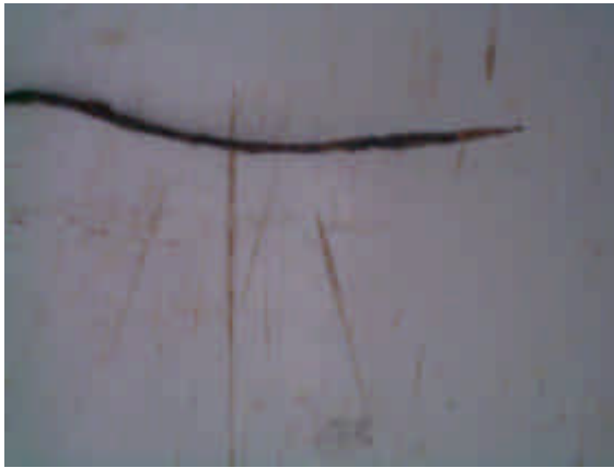
Photos showing the condition of the ground wire that was excavated from the existing structure. The ground wire from the ground line down, was corroded into 4 pieces.
