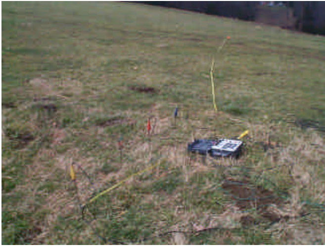
Line Traverse Method for Ground Resistance
