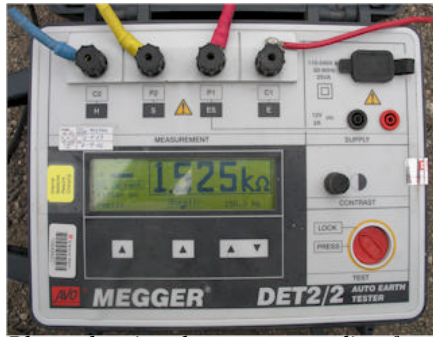
Photo showing the megger reading for the natively set pole. Megger reading is 1.525 K-Ohms or 1,525 ohms.
