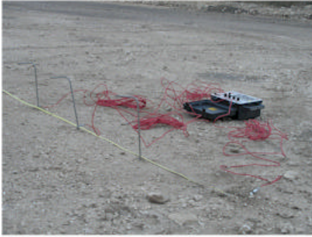
Photo showing Werner 4-Point Method for testing earth resistivity. The spacing was 2' in width representing a 2' depth. We could not get the probes deeper than the first incremental mark to go deeper so further evaluation was not possible. The 2' reading was 69 ohms but the reading was in essence inconsequential since no further readings were taken.
